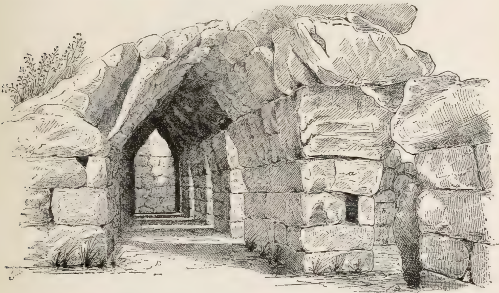
FIG. 78.—Perspective view of gallery of eastern wall. a , doors of chambers; b , partition wall of chambers.
